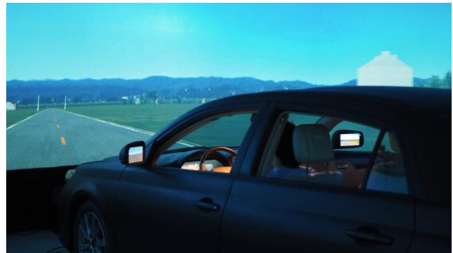
Figure 1. Driving simulator scenario built to represent a Level 3 autonomous vehicle
