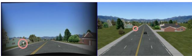
Figure 14. Front and aerial view of system biased towards false alarms brakes for all potential threats, including pedestrians on sidewalk who are not in the direct road path
