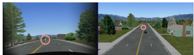
Figure 13. Front and aerial view of less sensitive system that does not detect and brake for pedestrians in opposing traffic lane
