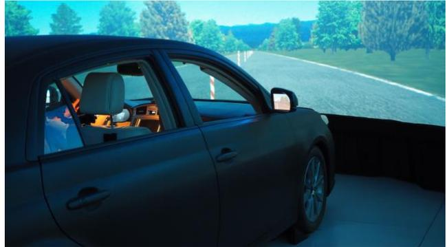
Figure 1. Full-vehicle driving simulator with programmed failure events
