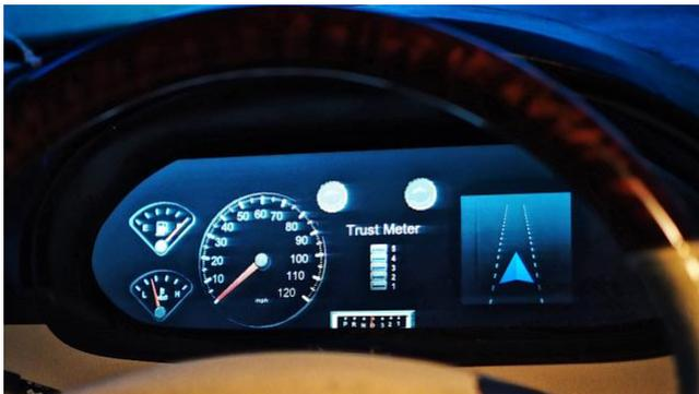
Figure 7. Trust meter indicator on instrument cluster, reflecting participants’ self-reported trust in system
