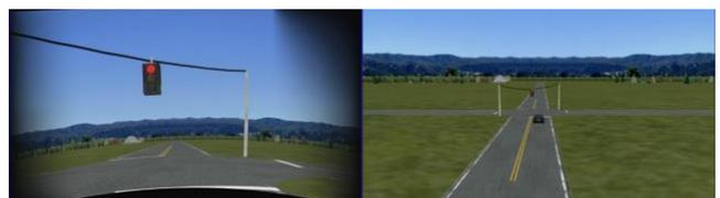
Figure 6. Front and aerial view of road as vehicle successfully slows down and brakes at a red traffic light
