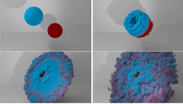
**Figure 2:** High-resolution smoke: Two spheres of smoke collide in a high-resolution 3D simulation ( $\Delta x = 1/255$ ). BSQLB accurately resolves vortical flow detail.
