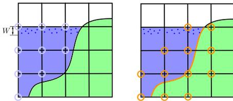
**Figure 11: Discrete free surface fluid domain.** *Left:* We define the fluid domain to consist of cells that either have (1) a particle (dark blue) in it or (2) a node with non-positive level set value (light blue). *Right:* Boundary Lagrange multiplier external pressure  $\lambda_b$  (orange circles) are like the interior pressures  $p_c$  except only defined on fluid domain cells that intersect  $\partial\Omega_S$ .
