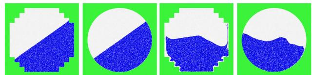
**Figure 15: Cut cell vs. voxelized domain.** Using a cut cell domain (right) instead of a voxelized domain (left) yields marked improvements in simulation quality.
