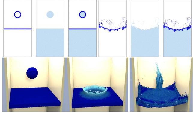
**Figure 12: Narrow band free surface.** A circle/sphere falls in a tank of water under gravity. Using only a narrow band of particles saves computational cost and enables increased resolution of the free surface. *Top:* In 2D we illustrate the hybrid particle (dark blue)/level set (light blue) representation. *Bottom:* Particles are colored based on velocity magnitude.
