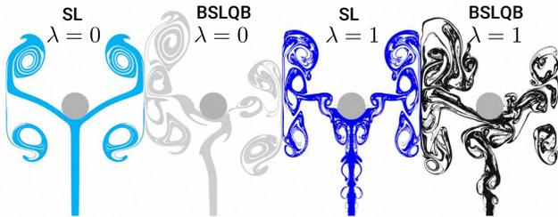
**Figure 16:** Interpolation correction. BSLQB exhibits more fine-scale flow detail and vorticity than semi-Lagrangian for extremal values of interpolation parameter  $\lambda$  (Equation (16)). From left to right: semi-Lagrangian with  $\lambda = 0$ , BSLQB with  $\lambda = 0$ , semi-Lagrangian with  $\lambda = 1$ , BSLQB with  $\lambda = 1$ .
