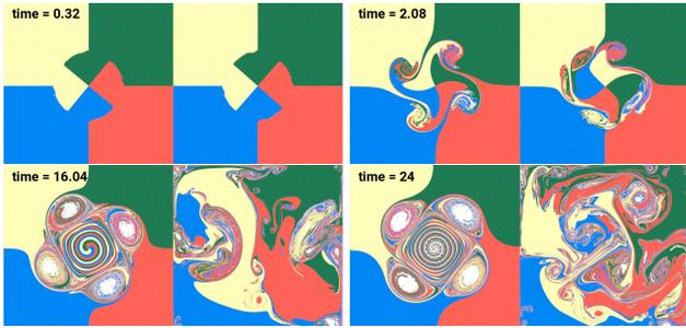
**Figure 6:** *SL vs. BSLQB.* We compare semi-Lagrangian (left) and BSLQB (right) in a vorticity-intensive example. BSLQB breaks symmetry and exhibits a more turbulent flow pattern. Note we only use particles for flow visualization and not for PolyPIC advection in this example.
