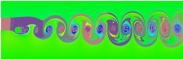
**Figure 14: Von Karman vortex shedding.** We demonstrate the accuracy of our Hybrid BSLQB/PolyPIC with vortex shedding past a disk in 2D. Note the smooth transition between regions with particles (PolyPIC) and those without (BSLQB).
