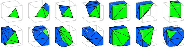
**Figure 13: Cut cells.** We show the 14 essential cases used in determining the cut cell fluid domain geometry. Blue faces indicate the intersection of the grid cell with the fluid domain. Green faces indicate the velocity boundary condition faces on  $\partial\Omega_S$ .
