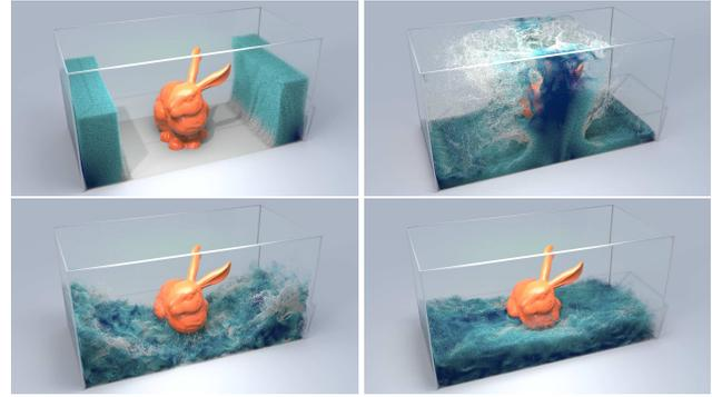
**Figure 5:** Dam break with bunny: Opposing blocks of water collapse in a tank and flow around the irregular domain boundary placed in the middle of the tank. Particles are colored from slow (blue) to fast (white) speed.
