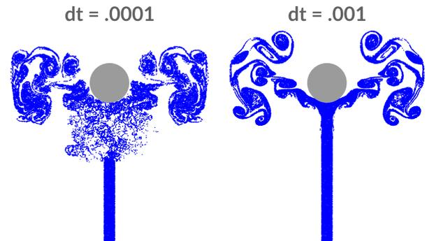
**Figure 20:** Instability: When  $\lambda$  is close (or equal) to 1, simulations can become unstable for smaller values of  $\Delta t$ . We show this here with a simulation of smoke against a circle at a spatial resolution of  $\Delta x = 1/127$ . This is seen for both semi-Lagrangian and BSLQB.
