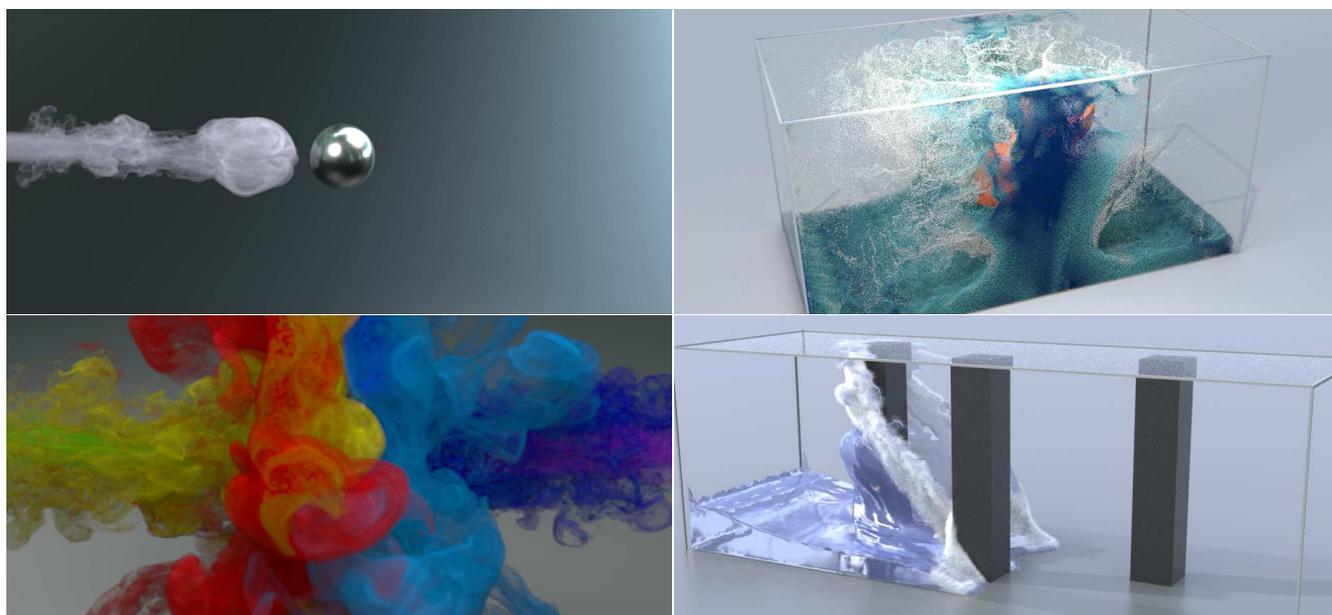
**Figure 1:** We simulate detailed incompressible flows with free surfaces and irregular domains using our novel hybrid particle/grid simulation approach. Our numerical method yields intricate flow details with little dissipation, even at modest spatial resolution. Furthermore, we use collocated velocity grids rather than staggered MAC grids.
