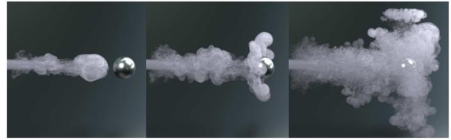
**Figure 18:** Smoke jet. A plume of smoke is simulated with BSLQB. Zero normal velocity boundary conditions are enforced on the irregular boundary of the sphere inducing intricate flow patterns as the smoke approaches it.
